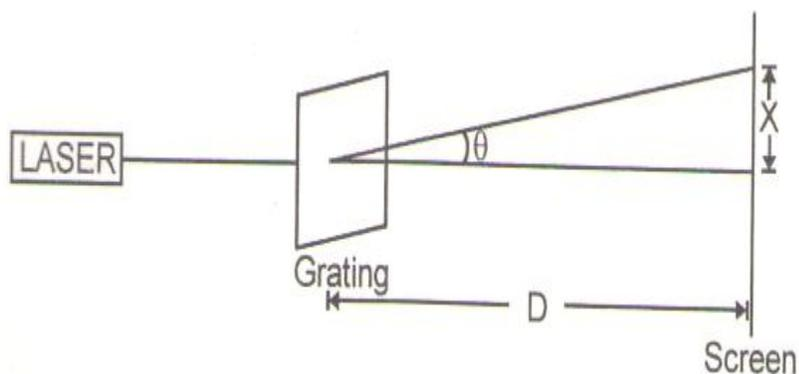
Fig.1. To determine the wavelength
